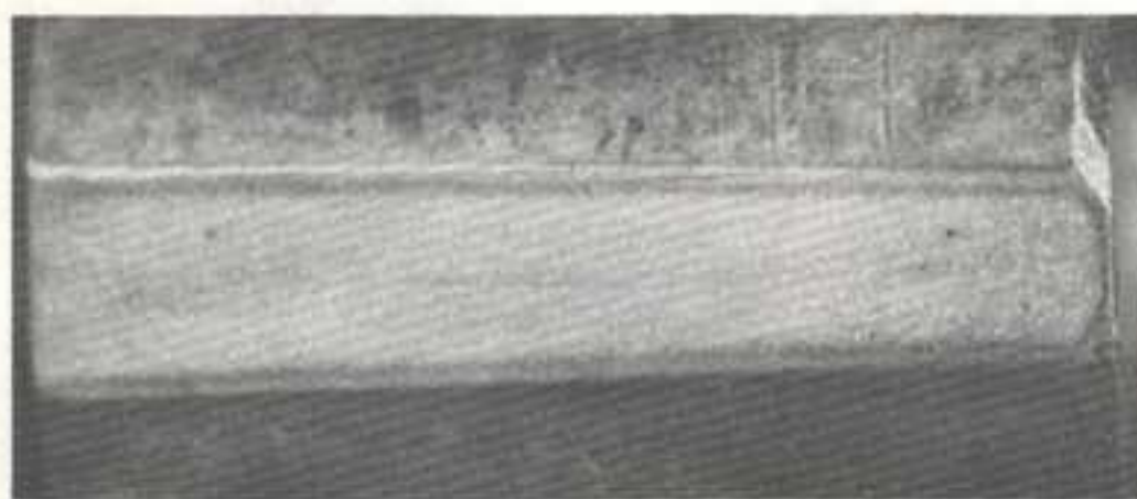
Fig. 38 This case-hardened pit has had a flat ground on the side and has then been etched to show the hardened case.
