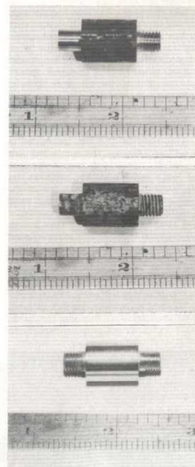
Fig. 37a Piece of M.S. prepared for carburising. 37b; After carburising, one end screwed and the other plain turned. 37c. The same piece after reheating and quenching. 37d; The plain end has been screwcut and the whole cleaned up. The bearing surface is dead hard, but both screwed ends are soft.
